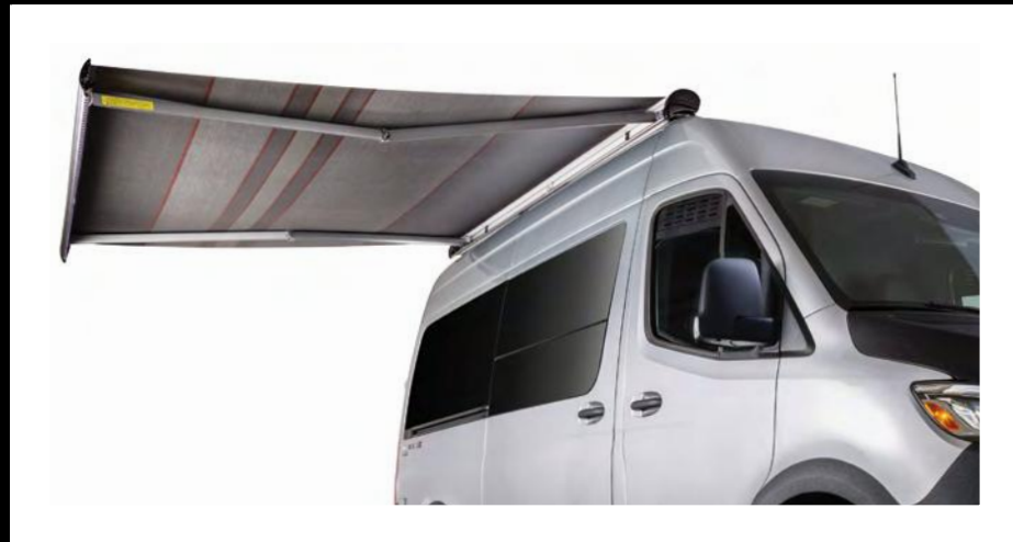
5 Powered armless patio awning extends with push-button ease.
